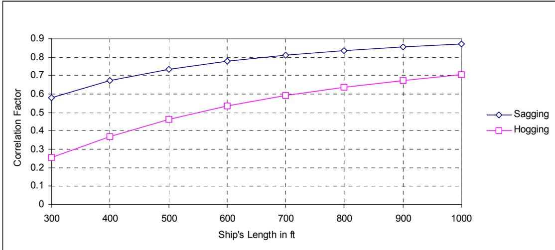
Figure 4. Correlation Coefficient of Whipping Bending Moment (kD)
