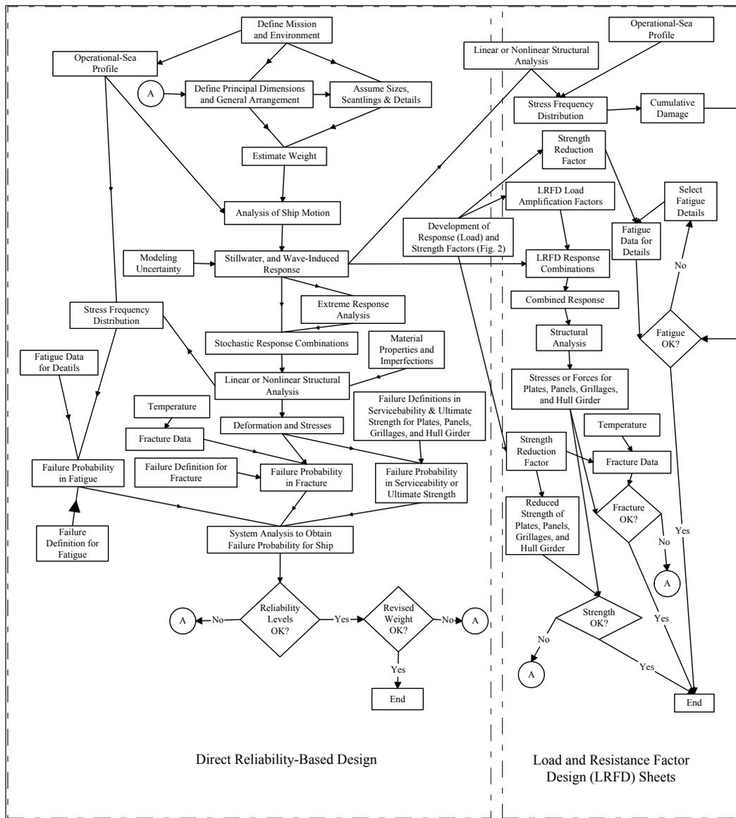
Figure 1. Reliability-based Design of Ship Structures (Ayyub et al 1998)
