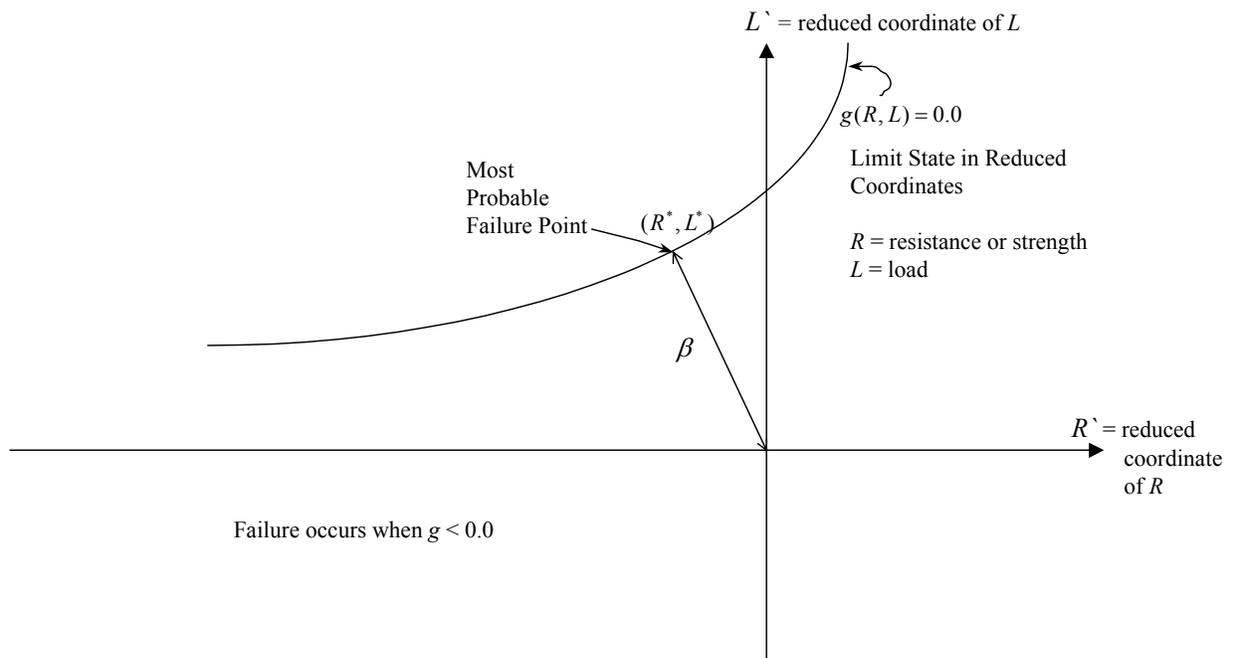
Figure 3. Space of Reduced Random Variables Showing the Reliability Index and the Most Probable Failure Point
