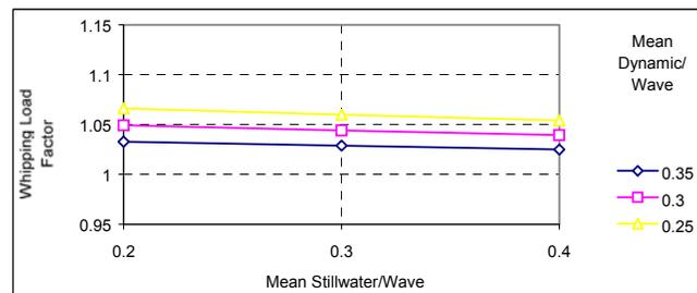
Figure 5. Variation of Strength and Load Partial Safety Factors versus Variation of the Ratios for the Mean Values of Load Components for the Example
