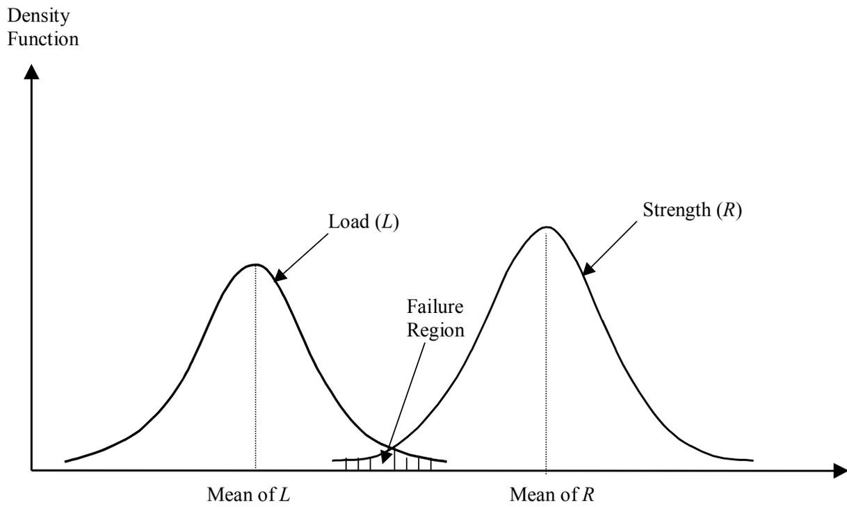
Figure 2. Frequency Distribution of Resistance  $R$  and Load  $L$
