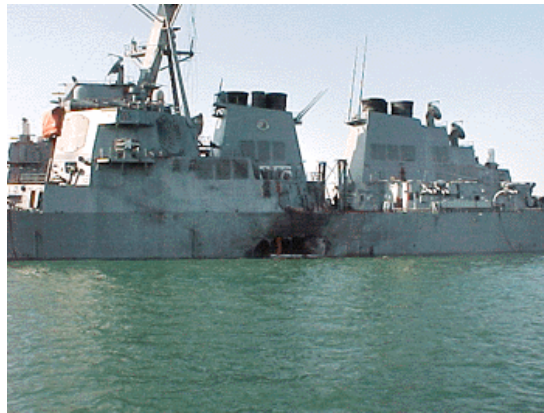
Figure 3. Port of Aden, Yemen, Oct. 13, 2000; USS Cole (DDG 67) After an Explosion on Oct. 12, 2000 which left a 40 foot by 40 foot Hole in the Port side of the Norfolk, VA-based Destroyer; Damaged Ship (U.S. Navy photos)
