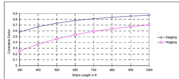
Figure 4. Correlation Coefficient of Whipping Bending Moment ( $k_D$ ) for  $300 < LBP < 1000$  ft (Mansour et al 1984 and Atua 1998)
