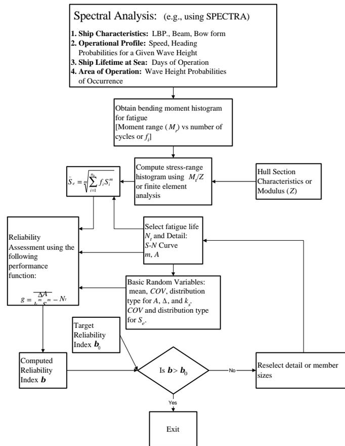
Figure 3. Direct Reliability-based Design and Analysis for Fatigue (Assakkaf, 1998)
