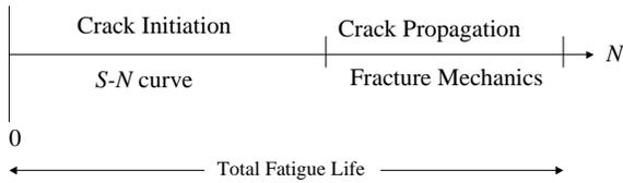
**Figure 1. Comparison Between the Characteristic S-N Curve and Fracture Mechanics Approach**
