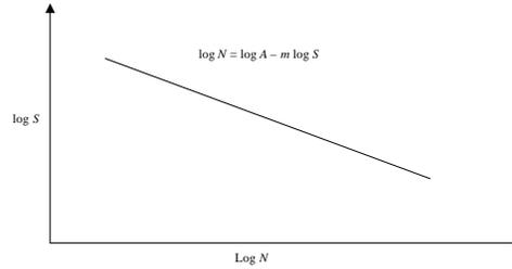
**Figure 2. S-N Relationship for Fatigue**
