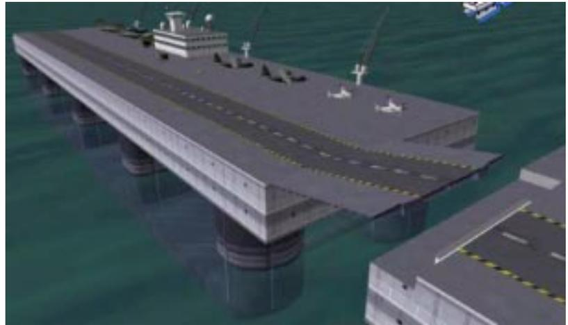
**Operational requirements for the MOB include the ability to support Air Force cargo aircraft, support container ships, provide massive storage of bulk and liquid stores, house 10,000 or more troops, and discharge various amphibious craft.**
