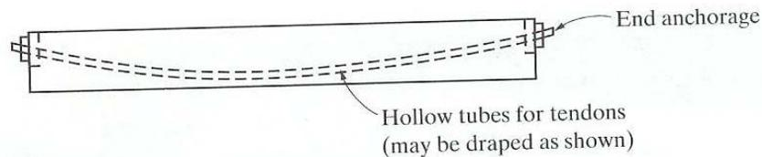
**Figure 3.** Post-tensioned Member
