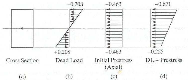
**Figure 4.** Midspan stresses for Example 1
